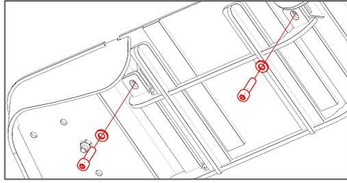
THEN TIGHTEN THE BOLTS HOLDING THE FOOTREST.
