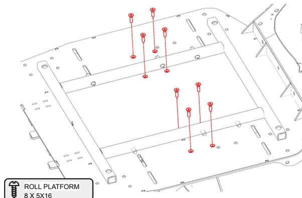
**13** PULL THE CABLES COMING OUT OF THE PITCH THROUGH THE HOLES ON THE TOP OF THE ROLL. INSERT THE CENTRAL SHAFT OF THE PITCH INTO THE HOLE ON THE TOP OF THE ROLL AND SCREW IT TOGETHER.
