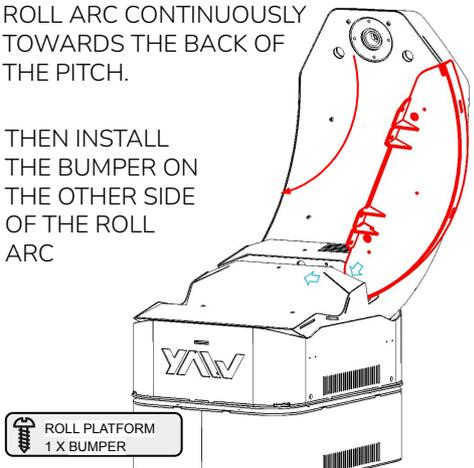
**12** MOUNT THE SIDE RAIL ON THE **ROLL** (OPTIONAL, STEP "A1"). THEN MOUNT THE ROLL ON THE ROLL ARC SO THAT THE "FRONT" SIGNS ARE ALIGNED TO EACH OTHER. SCREW TOGETHER AS SHOWN IN THE PICTURE
